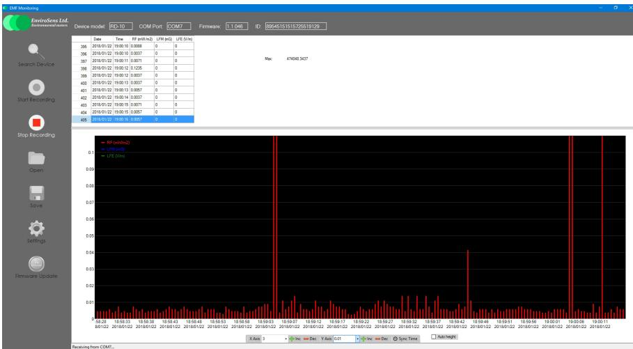
The **RD-10** software (which is a download) can be used to record and view readings from the Meter once it is connected to a PC using the supplied mini-USB cable.
